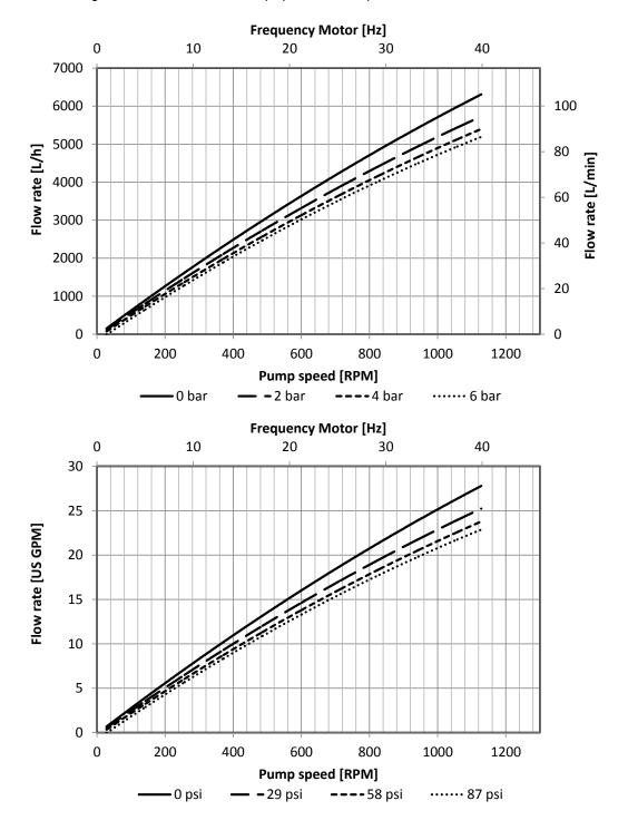
The flow rates showing at the charts above were ascertained with new diaphragms and new valves under standard conditions after the final assembly of the pump.
